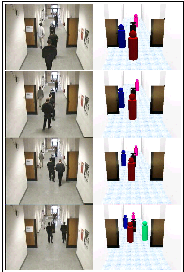
Figure 4. Tracking sequence showing a real photo and a 3D visualization of the state estimate at the same point in time. The time delay between consecutive images is 1.25 seconds.
